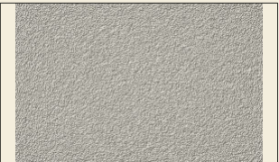
LW-2 Render, warm white Architraves, the frieze band, cornices, window hoods and the pediment tympana.
