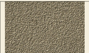
G-1 Courts and accessway, crushed granite Compacted granitic sand on a base course, all-weather (53.02-5 Table 3).
