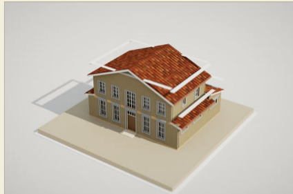
12 Eaves and porch linings Dressing: the architecture
